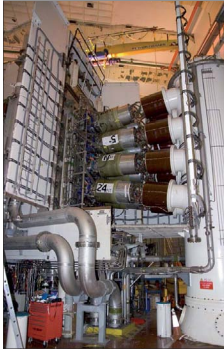
After the upgrade, JET’s neutral-beam injector will reach a test power of 34 MW.
