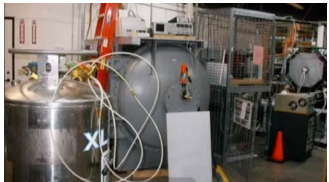
Figure 32 — Lab, View of Vacuum Tank
