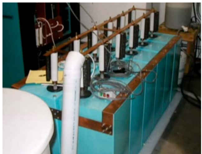
Figure 33 — Lab, Bank of 12 Capacitors providing 400K-joules at 15 Volts
